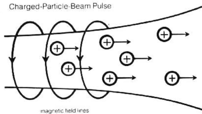
*Figure 4. A charged-particle beam will tend naturally to spread apart, due to the mutually repulsive forces between the like-charged particles constituting the beam. The electric current created by the moving charges will generate a surrounding magnetic field, which will tend to bind the beam together. However, unless there is some neutralization of the charge, the mutually repulsive force will always be the stronger force and the beam will blow itself apart.*
