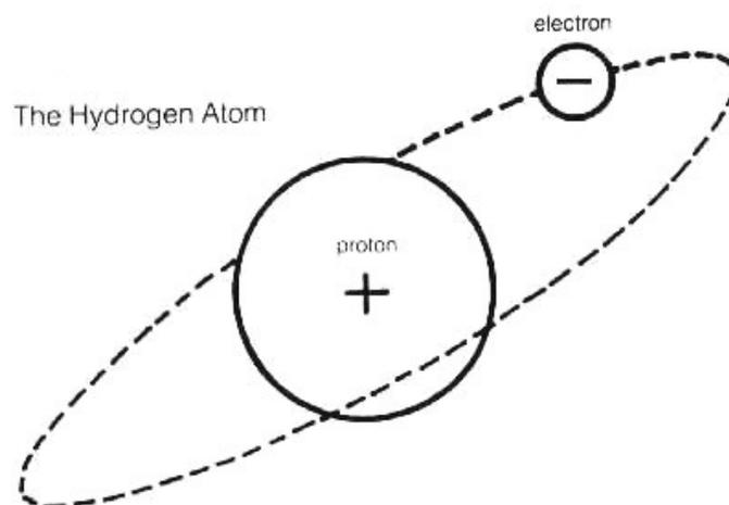
*Figure 1. The hydrogen atom consists of a proton or positive charge, orbited by an electron of equal but opposite (negative) charge. Together, they form a neutrally charged atom, which can serve as the "bullet" of a particle-beam weapon in space. Also, the proton and the electron themselves are both viable candidates as the ammunition for an endoatmospheric weapon.*
